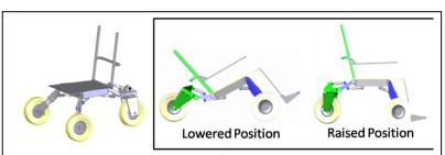
Fig.1: Advanced wheelchair frame design integrating tilt functions with dynamically controlled suspension
