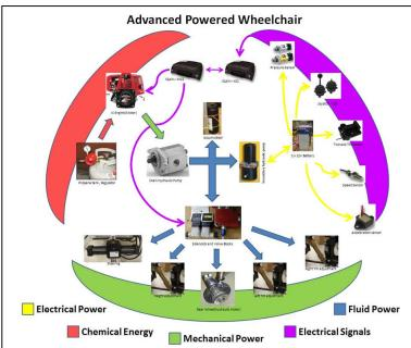
Fig.2: The engine powers the hydraulic system through a hydraulic pump and two controllers control the hydraulic system to move the wheelchair
